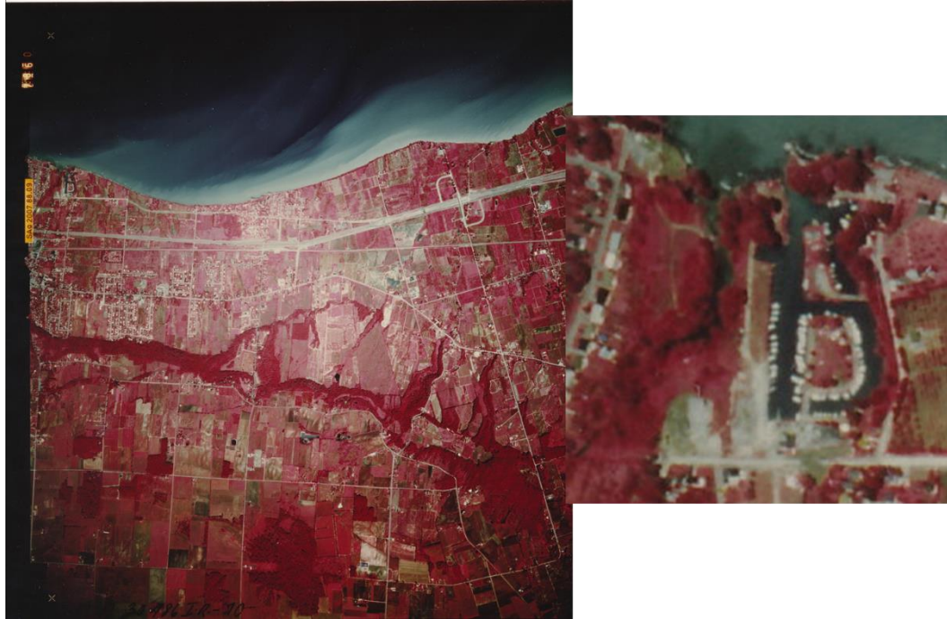
Figure 1a: Original image approximately 1:130,000 scale Colour Infrared Imagery of the sort used in the Great Lakes Land Use Mapping Project. The enlarged area shows the Grimsby Marina from the upper left corner of the full image. The detail was sufficient for identifying a variety of land use classes.
